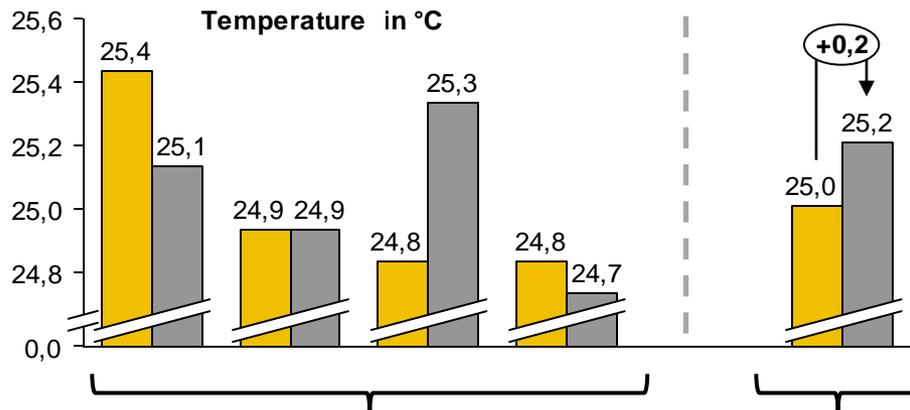
Comparison of simulation and measurement at some positions in the server-room. Deviation  $\pm 0,5$  °C
