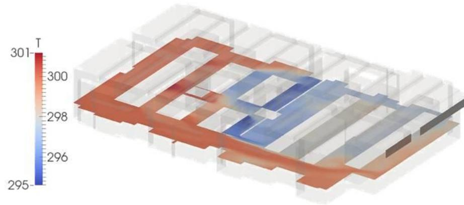
After adaptation of the separating wall with the suggested fans the temperature in the server room was monitored during a two day experiment.
